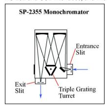
Figure 1. Includes a 90° optical path, Figure 2. Includes a 90° optical and micrometer adjustable entrance path, large 14 mm X 27 mm focal and exit slits.
